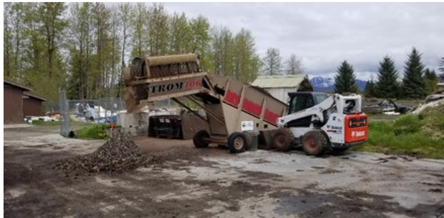
Compost screener - chips on the left, compost to the right
