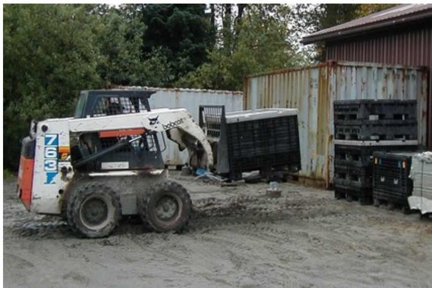
Bobcat skid-steer loader & collapsible pre-bale material storage bins
